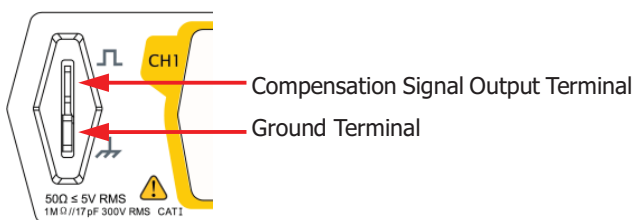
Figure 1-10 To Use the Compensation Signal
