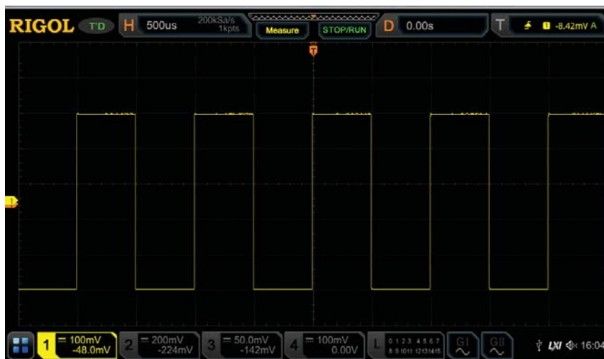
Figure 4-3 Waveforms after 128 Times of Averaging
