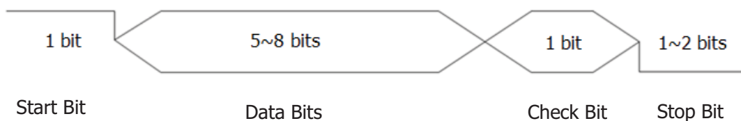
Figure 5-13 Schematic Diagram of RS232 Protocol
